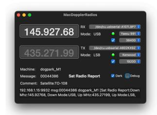
The MacDopplerRadios application takes the UDP output from MacDoppler running on the same LAN and translates the UDP messages into Radio commands for two separate radios, one uplink (TX) and one downlink (RX).
